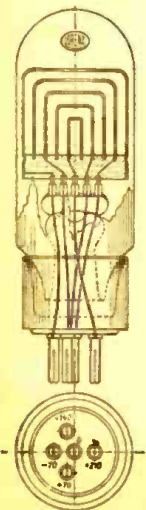
Fig. 1 At the left, a cross-section through the nested electrodes of the glow-tube voltage divider; it is so designed that a potential difference of 70 volts is maintained between each pair. Below, a diagram, showing how it is connected in a power-supply unit, with additional taps as needed.
